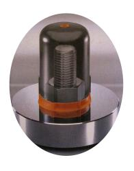
Protective Caps that feature a captive, soft sealing lip made from elastic, flexible material that adapts to suit the base of the nut, providing an excellent seal and guaranteeing a stable hold. These caps are especially suited for use on nuts and bolts in damp and off-shore environments, enhancing lifespan and running times of Plant and Machinery.
