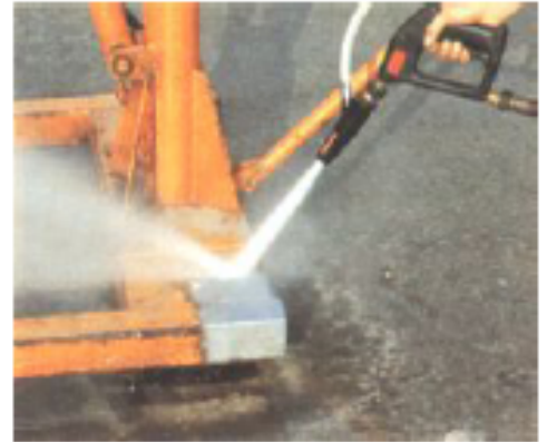
The water-sandblasting head TAIFUN feeds the blasting agent into the high pressure beam so allowing efficient de-rusting, paint removal and abrasive treatment of concrete surfaces, facades, etc.
