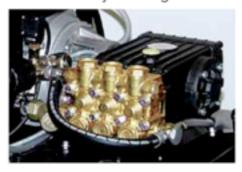
Fitted with smooth running, durable inline plunger pumps, these pumps have an excellent flowrate at a low pump speed.
