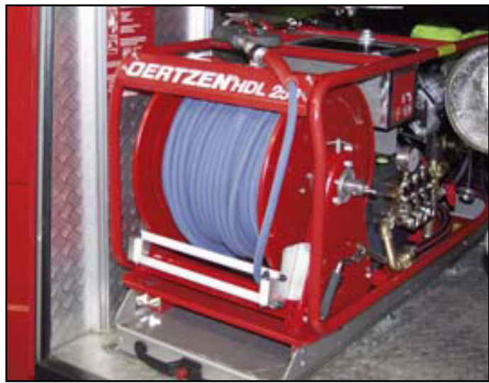
HDL-250 Installed - Closeup - 100m Hose
