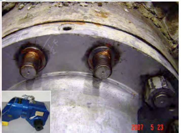
HY-25XLT™ HY-25XLT with 115mm Socket @ 16059 ft lbs being used by the Turbine Maintenance section
