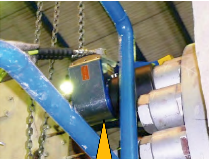
HY-25XLT™ HY-25XLT with 115mm Socket @ 16059 ft lbs being used by the Turbine Maintenance section
