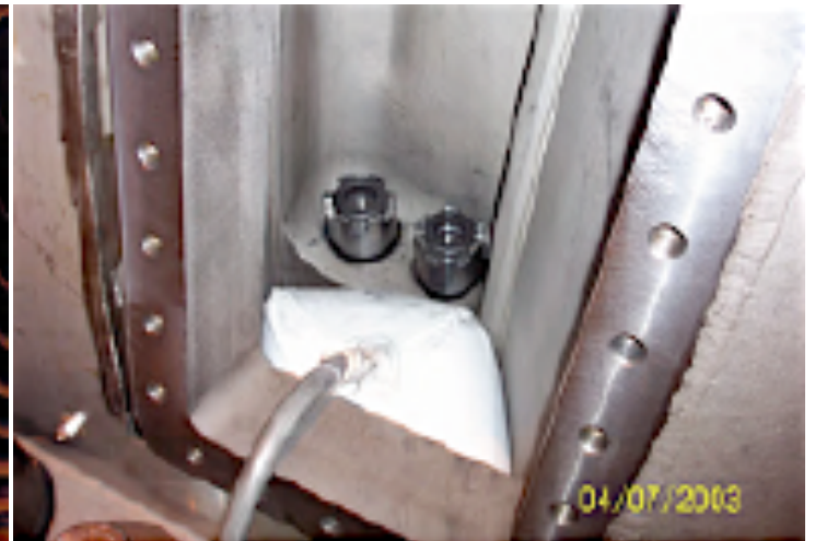
LOW PRESSURE- POCKET BOLTS (4Bolts)
