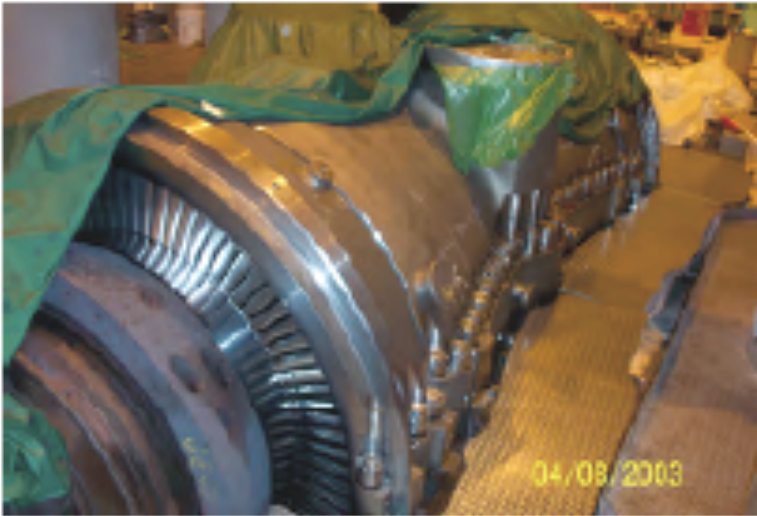
HIGH PRESSURE TURBINE (84Bolts)
